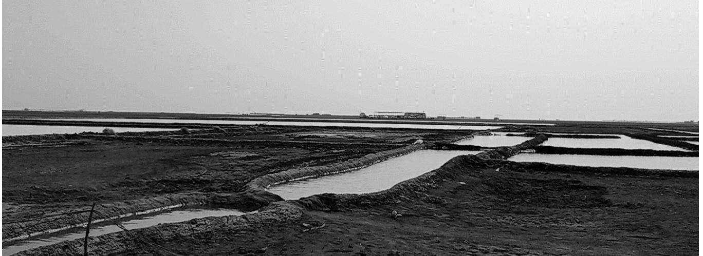
The salt pans connected through channels for the flow of brine to the crystalliser. The water has to pass through 23 pans before it reaches the crystalliser.
